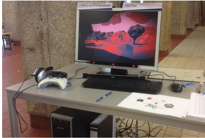
Figure 3: The employed setup consisting of a standard PC, a Tobii EyeX and a Tobii REX Eyetracker, an Xbox controller and headphones (Fractile game prototype).
