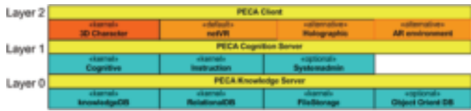
Figure 7: PECA Layered Architecture View
